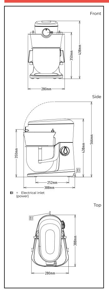
Electric Supply voltage: 200-240 V/1N ph/50/60 Hz **Electrical power max.:** 0.5 kW **Total Watts:** 0.5 kW Capacity: Performance (up to): 0.75 kg/Cycle Capacity: 5.5 litres Key Information: External dimensions, Width: 280 mm External dimensions, 388 mm Depth: External dimensions, Height: 438 mm **Shipping weight:** 15.6 kg Net weight (kg): 0.75 kg with Semi spiral **Cold water paste:** hook
